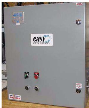
**Easy** Pump Control units are available for pumps of 1/2 to 20 horse power with power supplies of 230 volt single phase, 230, 460 and 575 volt three phase. Features include precise pressure control, gentle pump acceleration and deceleration with ASD, motor, and pressure safety protections.
